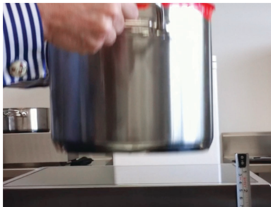
Heavy drop test on tough NEG glass*
