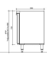
Ground Clearance Leg (standard): 130 to 165 mm Castor (optional): 95 to 115 mm Plinth (optional): 0 mm
