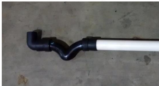
figure 17 drain trap orientation
