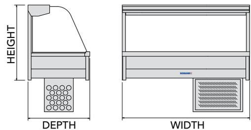
Note: For CRX model range overall height dimensions, add height of motor cage (450 mm).
