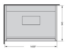
$\pm$  15 mm adjustable feet For transport the depth can be reduced to 870mm
